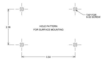
Fig. 2: Hole Pattern for Surface Mount
