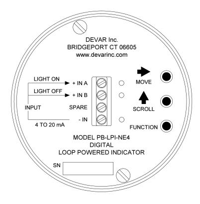
Fig. 5: Back of Display Board
