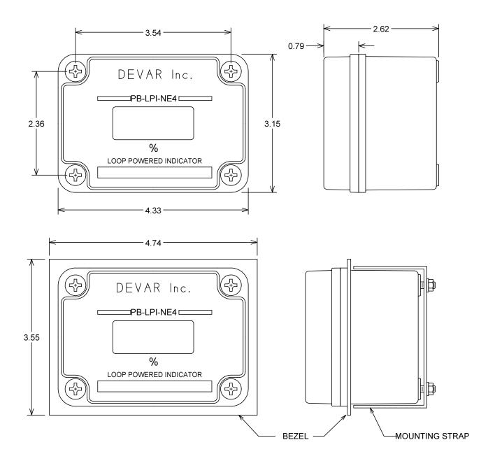
Fig. 3: Option -M46 NEMA-4 Panel Mount Dimensions
